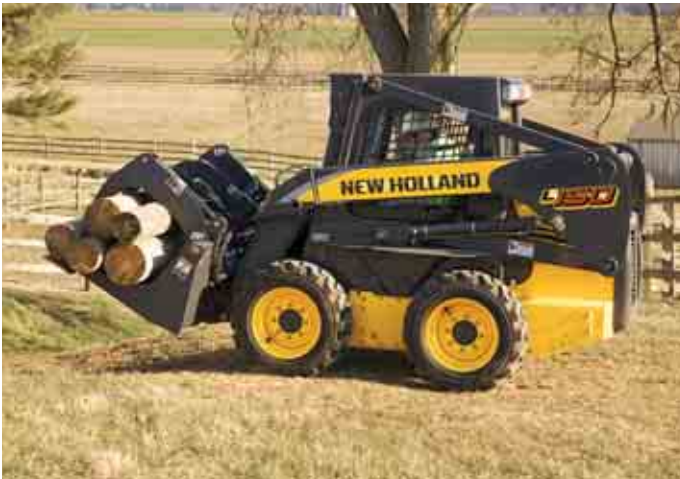
L150 is shown with the grapple attachment.
