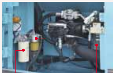
Main fuel filter Pre-fuel filter (with built-in water separator) Engine Oil Filter *Optional for NZ
