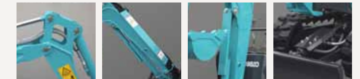
Bucket cylinder hose inside the arm Hose protection cover on back of boom Boom cylinder protection cover Dozer cylinder protection cover
